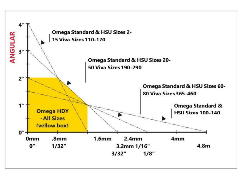
**NOTE:** Omega Standard Orange, Omega HSU, and Viva maintain their service life for any combination of parallel and angular misalignment measurements which fall on or below the line of the respective size. For Omega HDY, permissible misalignment values are shown in the yellow region and below the corresponding coupling size dotted line.
